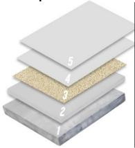
CrownCrete-U<sup>™</sup> 838 TG Urethane Mortar and a Single Broadcast of Natural Quartz Mil (4.75 mm), 7521 CrownPro<sup>™</sup> AcidShield<sup>™</sup> Novolac Epoxy Grout Coat and Top Coated Pigmented Flooring System, 3/8 Inch.
