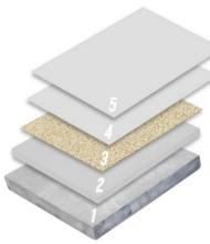
CrownCrete-U<sup>™</sup> 838 TG Urethane Mortar and a Single Broadcast of Natural Quartz Mil (4.75 mm), 8175 CrownPro<sup>™</sup> Polyaspartic Pigmented Grout Coat and Top Coat Flooring System, 3/8 Inch.
