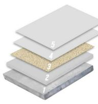
818 CrownCrete-U<sup>™</sup> Urethane Mortar and a Single Broadcast of Natural Quartz 187 Mil (4.75 mm), 8175 CrownPro<sup>™</sup> Polyaspartic Pigmented Flooring System, 3/16 Inch.
