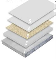
818 CrownCrete-U<sup>™</sup> SL Urethane Mortar and a Single Broadcast of Natural Quartz 187 Mil (4.75 mm) and Top Coated with 810 CrownCrete-U<sup>™</sup> SC (Skim Coat) Pigmented Flooring System 3/16 Inch.
