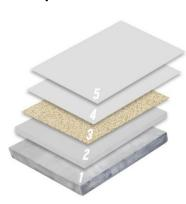
818 CrownCrete-U<sup>™</sup> Urethane Mortar and a Single Broadcast of Natural Quartz 187 Mil (4.75 mm), with 8320 CrownShield® Chemical Resistant Pigmented Flooring System, 3/16 Inch.
