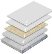
CrownCrete-U<sup>™</sup> 814 CrownCrete-U<sup>™</sup> Urethane Mortar and a Single Broadcast of Natural Quartz 250 Mil (6.35 mm), with 7521 CrownPro AcidShield Novolac Pigmented Flooring System, 1/4 Inch.
