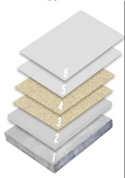
CrownCrete-U<sup>™</sup> 838 TG Urethane Mortar and a Double Broadcast of Natural Quartz 500 Mil (12.7 mm), 8320 CrownShield® Receiving Coat and Natural Quartz Aggregate, 8175 CrownPro<sup>™</sup> Grout Coat and Top Coat Pigmented Flooring System, 1/2 Inch.
