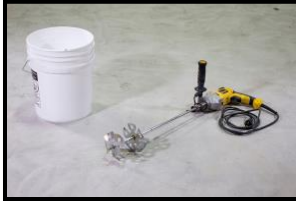
LOW SPEED HIGH TORQUE DRILL WITH EXTRA CORDS, & 5-GALLON BUCKET FOR MIXING
