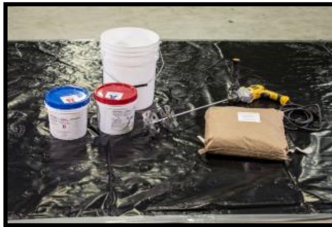
EXAMPLE OF A TYPICAL MIXING STATION SET-UP
